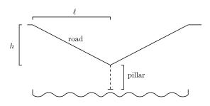
which lets us save on the costs of building the pillar. The resulting bridge costs A dollars per meter of paved road, plus the central pillar costing B dollars per meter of height. Given the constants  $\ell$ , A and B, we want to determine the ideal height drop h for the bridge.
