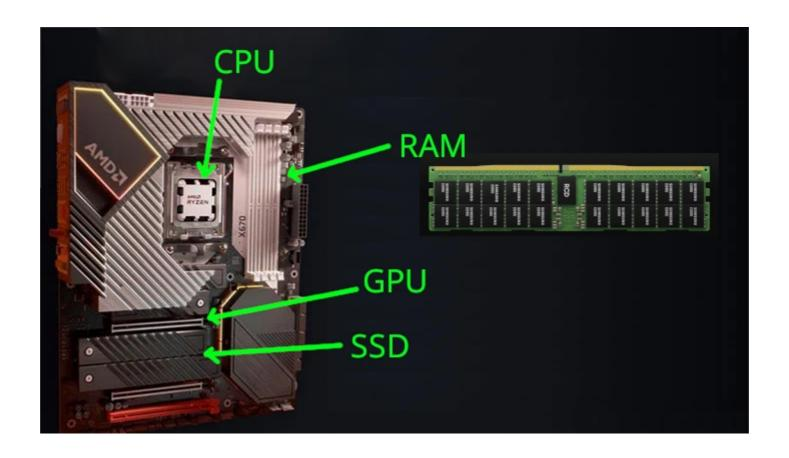
On desktop computers, RAM is typically on distinct integrated circuit (IC) packages, physically centimeters away from the CPU.
